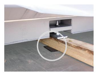
The two wooden planks must be wider than the machine to improve its stability.
